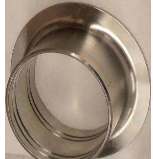
4-in sleeve for fiber potting
