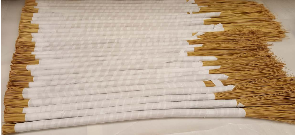
Photograph of 5000 fibers (5 m 2 ) arranged for potting at SRI
