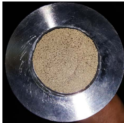
Potted 4-in fiber module cross-section (early design)
